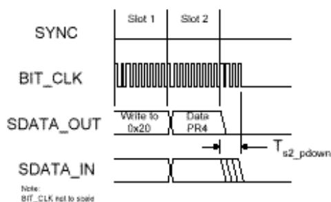
Fig 6.2.6-1 AC-Link low power mode timing diagram
