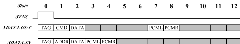
Fig5.2-2 ALC100 slot arrangement – CODEC ID = 10
